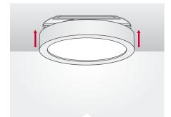
STEP 5: Push and feed all wires up into junction box as you raise the fixture into place. For wet location usage, please caulk the edge of fixture with glue to ceiling.
