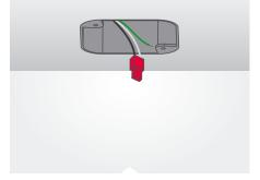
STEP 1: Turn-off / disconnect power at circuit braker. Attach orange connector (provided) to AC cable from junction box: L side to Black side wire. N side to White AC wire.
